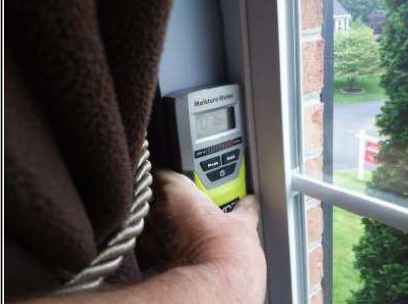
Moisture readings in the window openings are 76%
