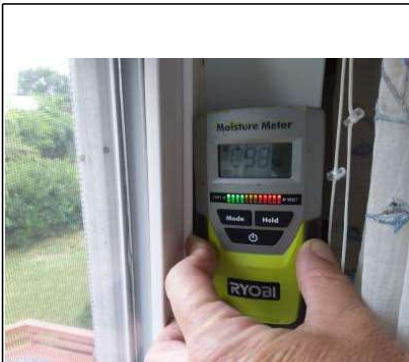
Moisture reading in the right window opening is 98%.
