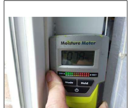
Moisture in the window opening is measured at 78%
