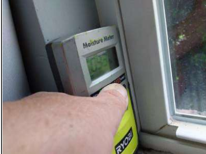
Moisture in the window opening is 93%.
