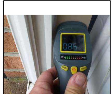
Moisture reading on the other window is at 85%.
