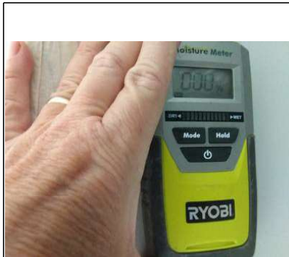
Moisture reading on the flat wall is 0%
