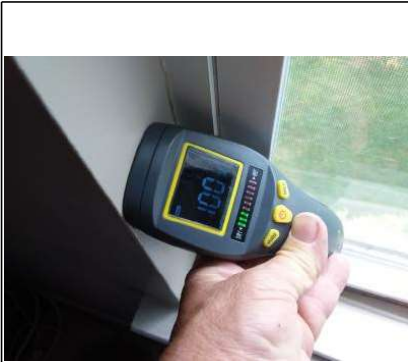
Moisture reading in the window openings at 100%.
